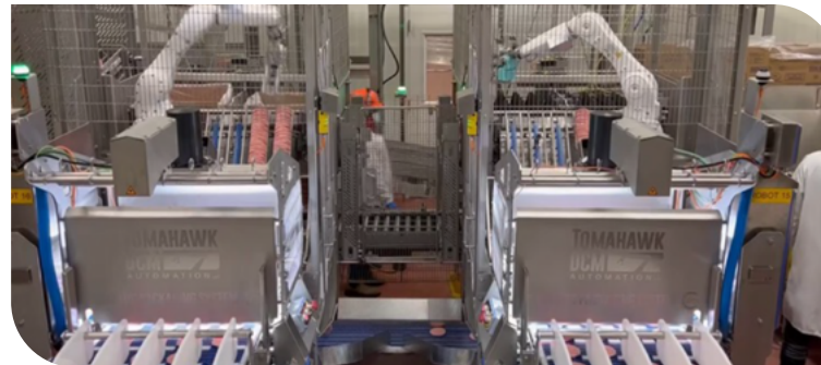
Patty-packaging robotics in use at Protein Products facility in Opelika, Alabama.
